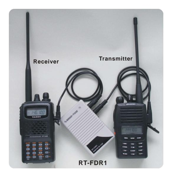
This picture just shows the connection of Receiver, Repeater Controller and Transmitter. For real repeater system, the antennas of both receiver and transmitter must be extended and installed for approximate 10 meters, or use a DUPLEXER to combine the RF signal of receiver and transmitter. These are the ways to provide adequate rejection of strong transmitter signal occurring at the receiving signal.
