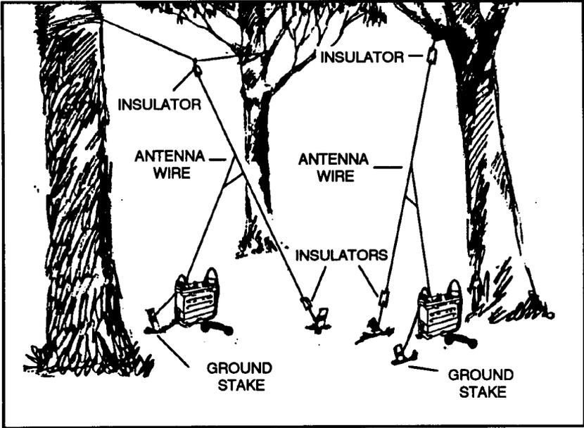
Figure 7-8. Improvised vertical half-wave antenna.
