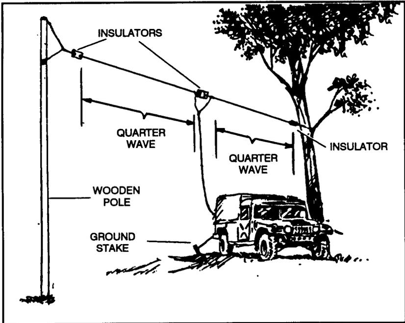
**Figure 7-6. Center-fed half-wave doublet antenna.**
