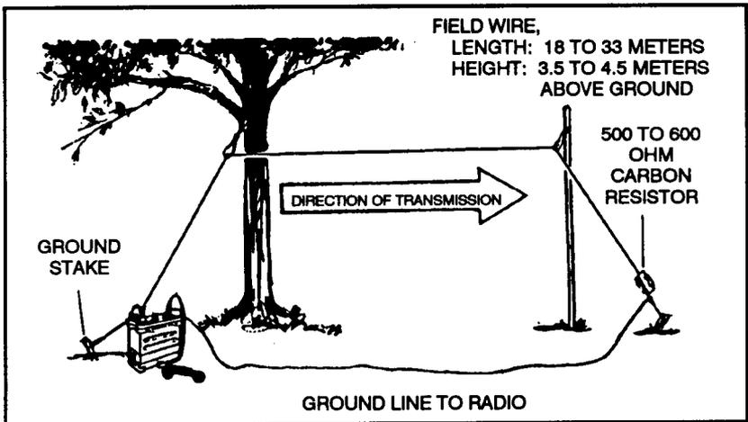
**Figure 7-10. Long-wire antenna.**
